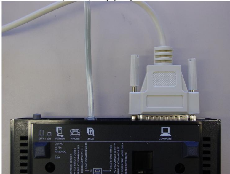
Figure 1-1. Modem connections to the computer's serial port and iridium phone line.
